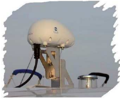
The Thorium™ – CLS' Iridium-based LRIT terminal
